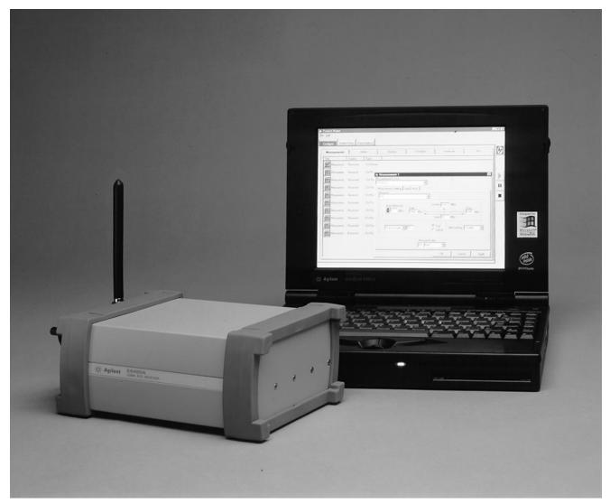
The Agilent Technologies E7450A RF coverage measurement system is used to obtain measurement versus location data to test the coverage of PCS communications networks. The E7450A system includes PC software, an E6450A PCS receiver, a cigarette
